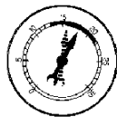
POOR VALVE SEATING AT IDLE
