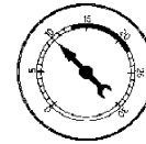
LATE VALVE TIMING, VACUUM LEAK AT IDLE
